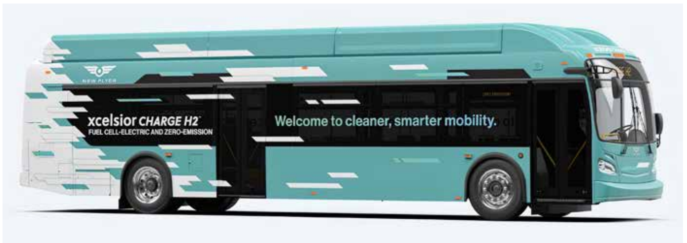
The New Flyer Xcelsior CHARGE H2™ is a battery-electric vehicle that uses compressed hydrogen as an energy source.
